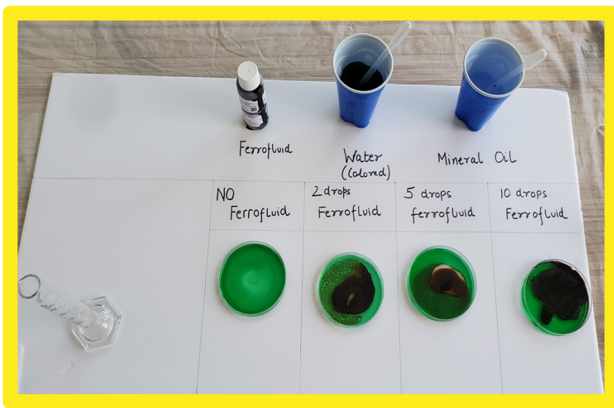
Figure 5. Place 2 drops, 5 drops and 10 drops of ferrofluid in the middle of the oil spill in the petri dish in the "2 drops ferrofluid" column, "5 drops ferrofluid" column and "10 drops ferrofluid" column respectively
