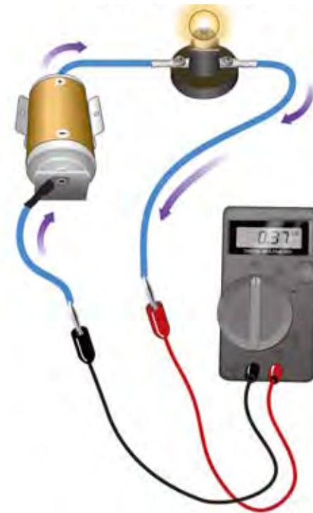
Figure 20.12: Current must pass through the meter when it is being measured.
