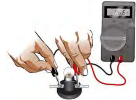
Figure 20.17: A multimeter can be used to measure resistance of a device.
