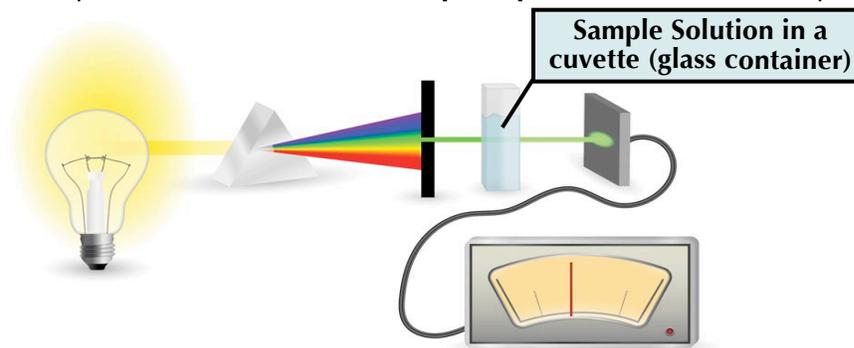
**How a Spectrophotometer Works =**
