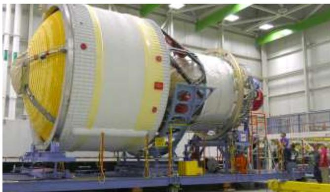
For Artemis 1, the interim cryogenic propulsion stage provides the power to send Orion 280,000 miles from Earth and 40,000 miles beyond the Moon, farther than any spacecraft built for humans as ever traveled.
